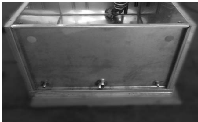
Side fixing points for discharge solenoid valve and 1/2" float valve
