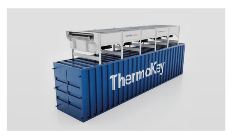
Dry Coolers with single cooling circuit designed and manufactured to perform at high ambient temperatures (max 60°C) with high temperature inlet fluid (100°C). The ambient air is sucked in by the fans on the lower side of the finned pack and forced to pass through the finned heat exchanger. The air, therefore, after passing the engine, absorbs the heat from the cooling fluid preserving the fan life. This configuration prevents the fan motor from being run
