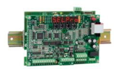
The EC PLUS Ep is a multifunction and multiple-input unit for the regulation of speed of threephase electronically commutated motors installed on axial fans, which is designed to regulate different EC motors, in a simultaneous and coordinated way, using programmable input signals. Power supply: IP55: 2ph+PE 400Vac ±20% (other voltages upon request)
