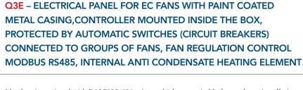
Metal casing painted with RAL7035, 120 micron thickness, suitable for outdoors installation.
