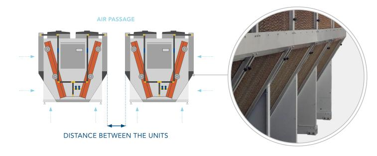
The sloping V-Tower solution saves space when there are more than one unit next to one another without reducing the operating efficiency.
