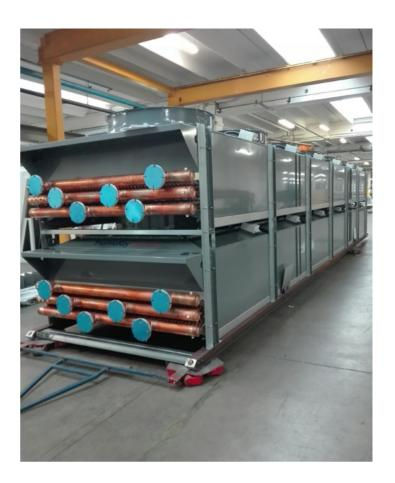
Cooling radiators for Rolls Royce engine - capacity 1665KW for HT circuit - 980KW for LT circuit
