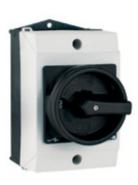
220-690V 20A - 3 poles Switch mounted and wired near to the fan Working temperatures -25°C ÷ 40°C Locked in the open position with padlock(OPTIONAL) Red handle (black only in presence of mainswitch) Protection class IP65 N°4 inlets Ø M20 Execution in compliance with CE regulations.
